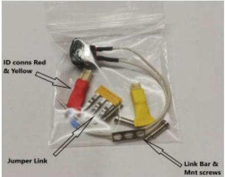
The Jumper Link should be fitted to inputs #15-17 (PIR) & the Link Bar should be fitted to inputs #18-20 (External switch).
